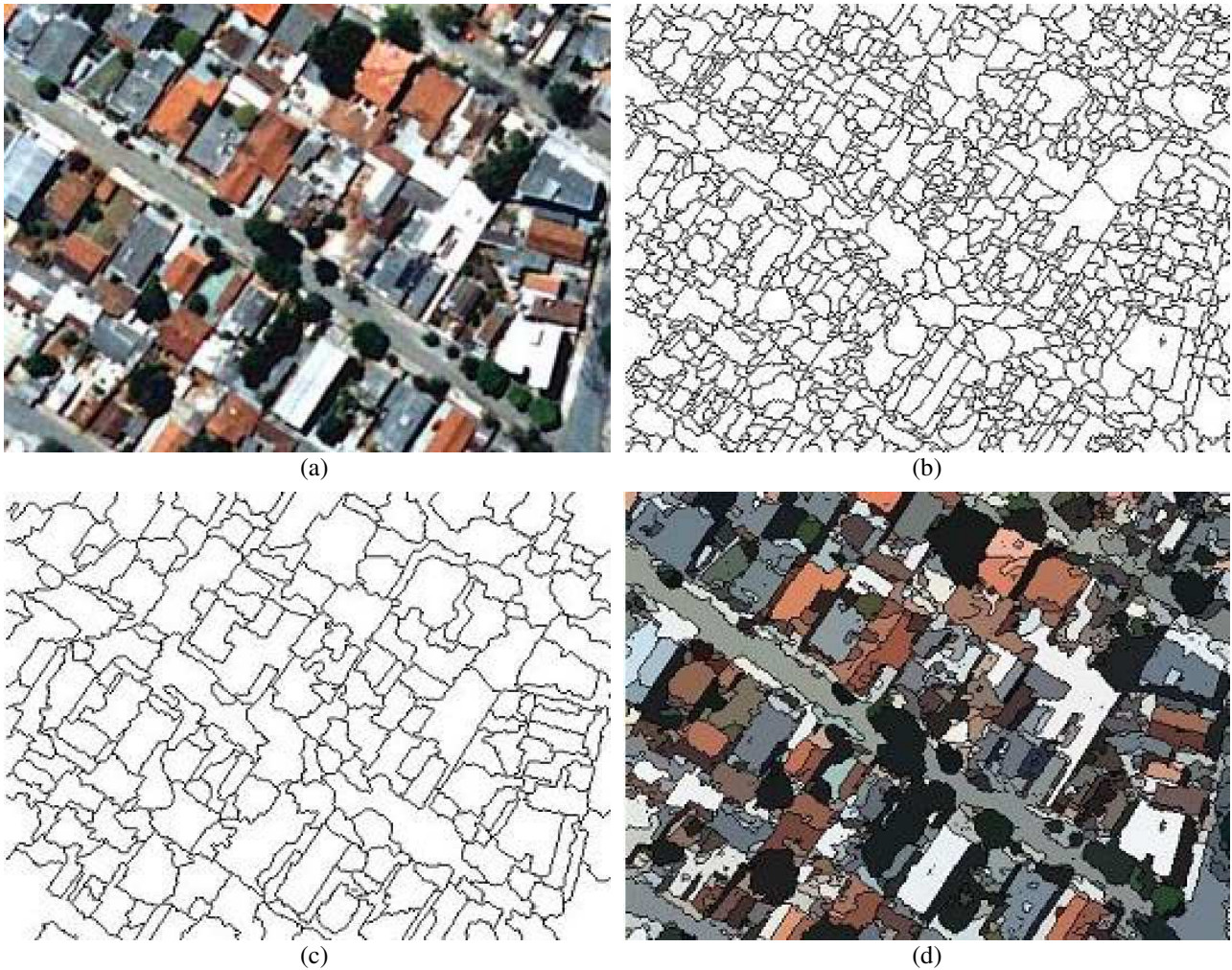
Figure 3. Watershed segmentation results. (a) Input image, (b-d) results with a small volume threshold, with a large volume threshold, and with combined volume and color thresholds, respectively.
