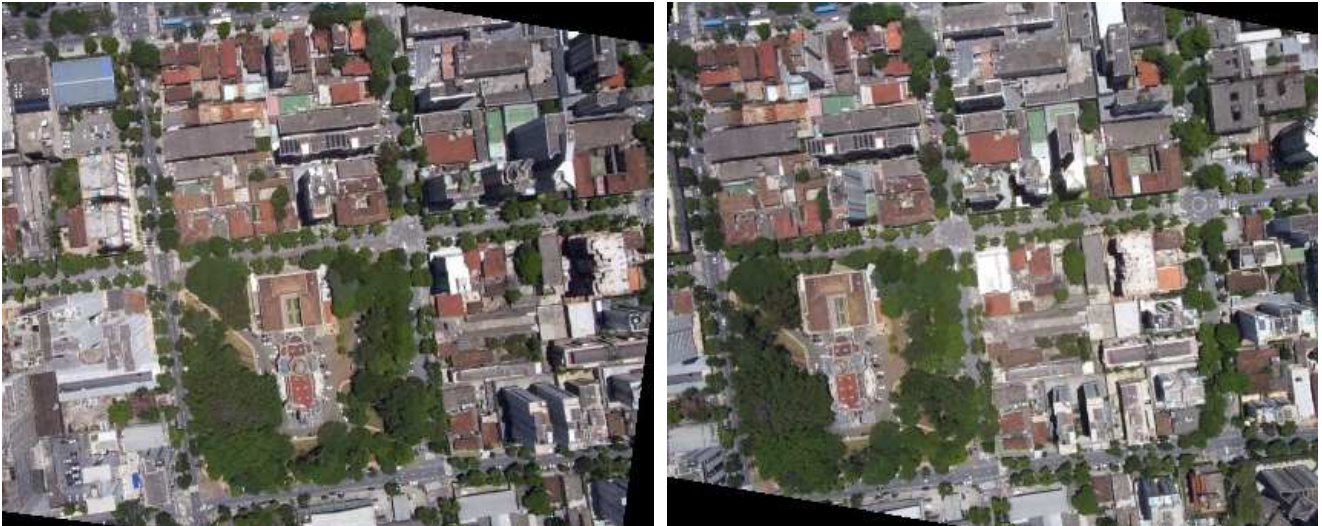
Figure 1. Rectified stereo pair created from shots taken 4 seconds apart in a low-altitude flight (1,500 feet relative to the ground) performed over the city of Belo Horizonte, MG, Brazil.
